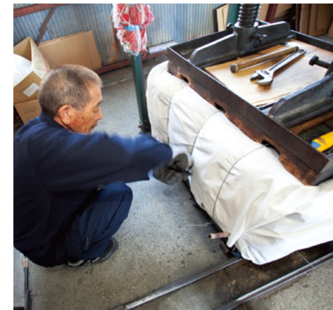
After sorting, special equipment is used to compress the clothes into compact bundles. Each package is then wrapped in tough cloth and tightly bound with thick wire.
